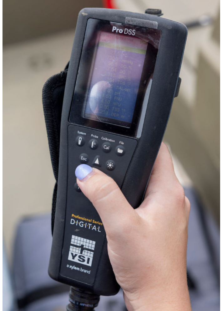
The CPN Environmental Department keeps a close eye on local water quality using a water quality sonde.
